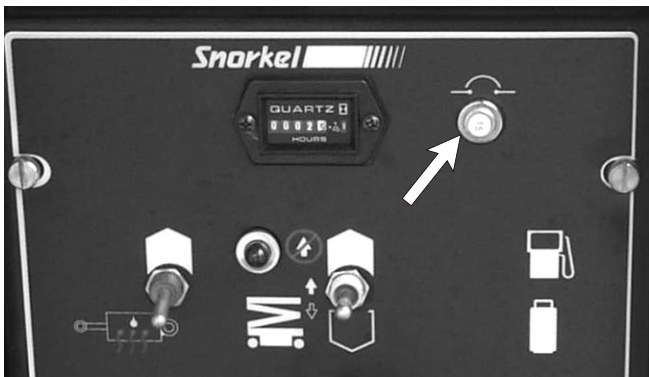
Figure 5.4 - Main Circuit Breaker
