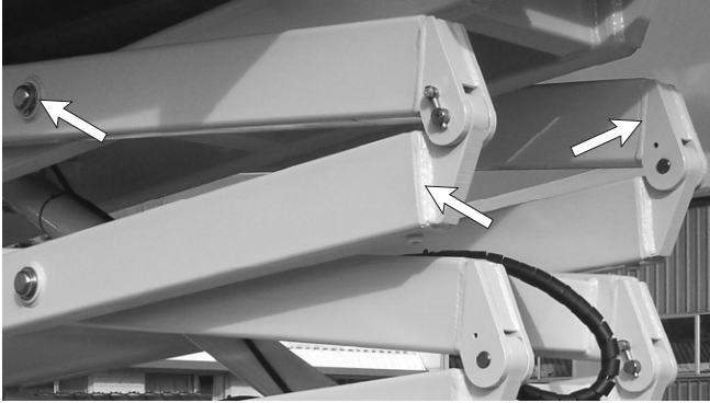
Figure 7.19 - Structural Damage and Welds
