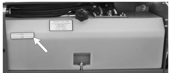
Figure 4.4 - Hydraulic Oil Level
